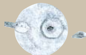
Peeled solder on the diode lead
