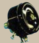
Exhaustion of grease in the volume resistor
