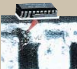
Short circuit due to the run-off of IC pin coating material
