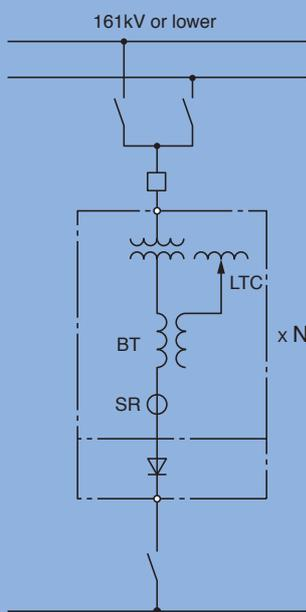
Fig. 10 Voltage control system, with 12 pulse rectifier units
