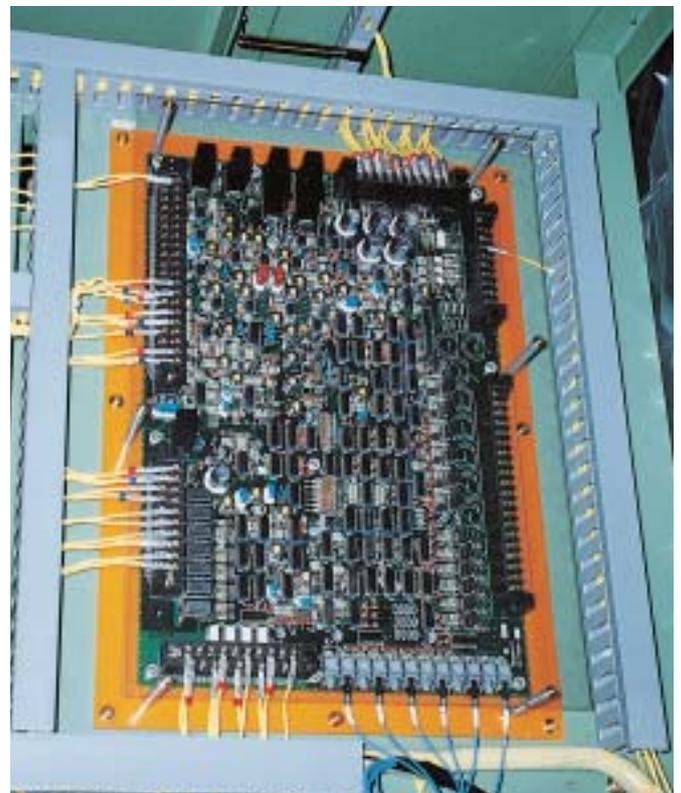
Automatic current control unit for thyristor rectifier
