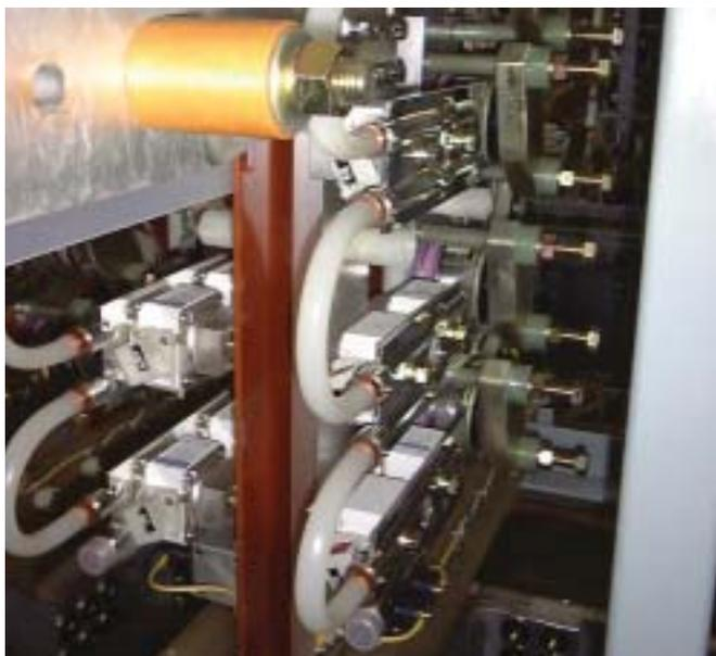
Water cooled heat sinks and diodes
