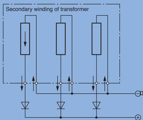
Fig. 6 Simplified in-phase contra-polarity Star connection
