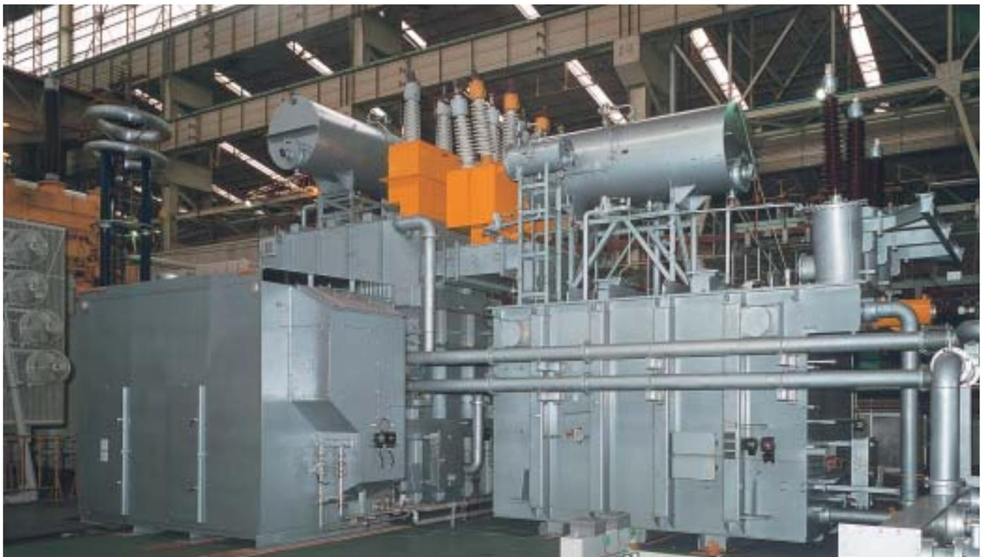
S-Former for outdoor installation, 1,330V DC, 85kA, 113.05MW
