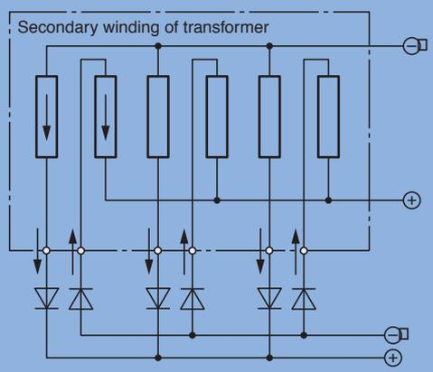
In Fig. 5, the secondary bushings of the transformer are positioned close to each phase, and the star connection is made outside of the transformer tank. Only local heating near the secondary bushing is reduced with this construction.
