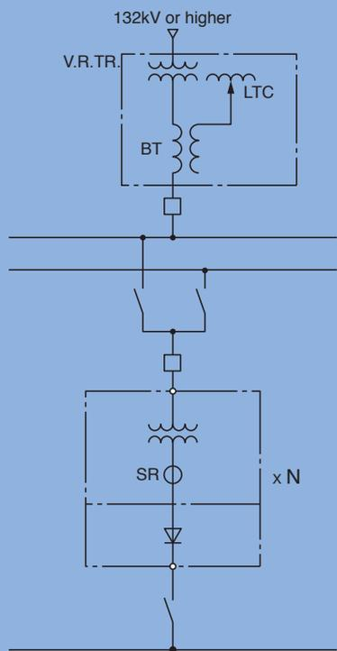
Fig. 9 Voltage control system, with 6 pulse rectifier units
