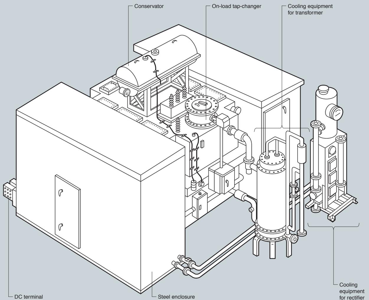
Note : Typical OFWF cooled transformer and WFWF cooled diode rectifier
